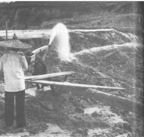
Plate 6 —Gravel pump tin mining involves the use of a monitor which jets water out to knock down tin-bearing soil.
