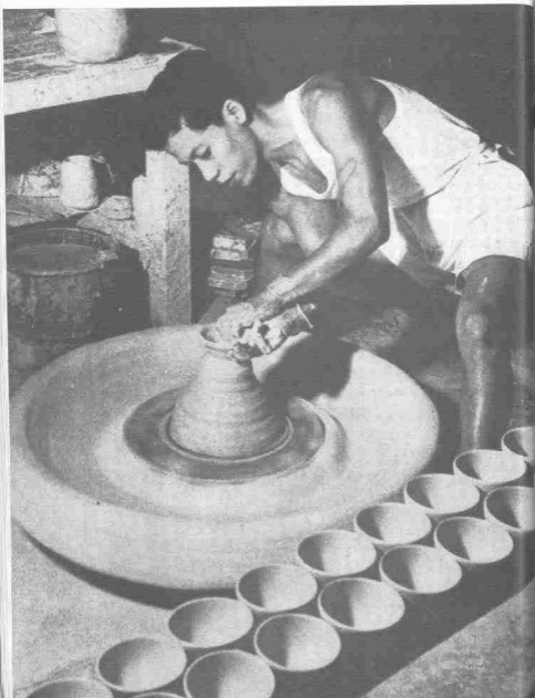
Plate 2 —In Malayan pottery locally mined China clay and lime are used. Picture shows a Chinese at work on the heavy potter's wheel shaping the latex cups with his skilful fingers.
